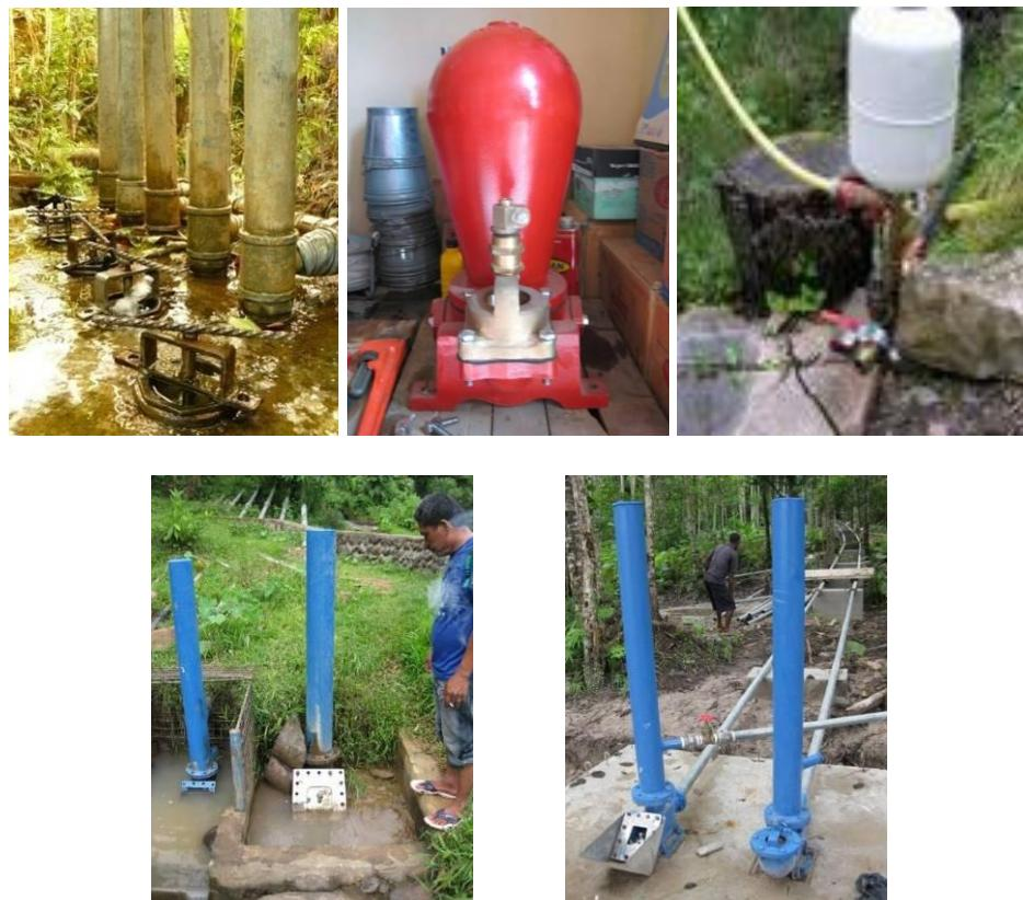
Figure 10: Example of Hydraulic Ram Pumps around the world
