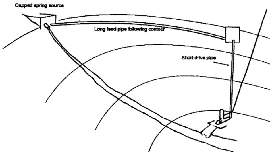
Figure 18: Topography and drive pipe position
