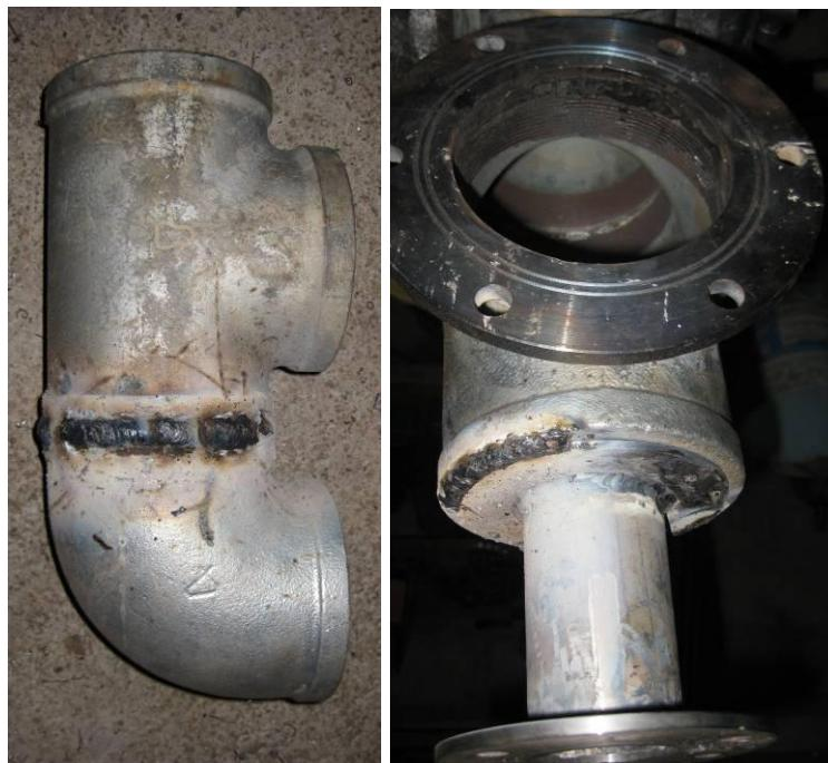
Figure 30: Welding the pump body
