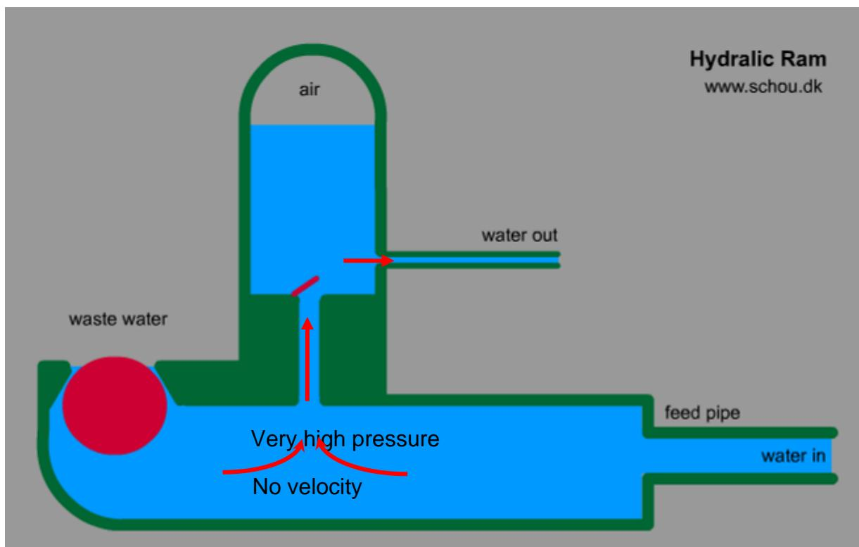
Figure 3: Application of the water hammer effect on the Hydraulic Ram Pump
