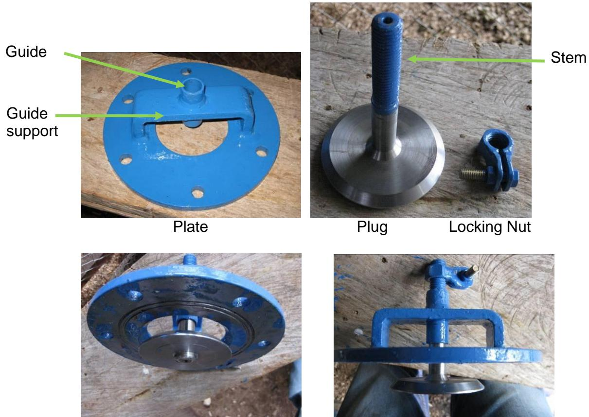
Figure 13: Impulse valve and its components
