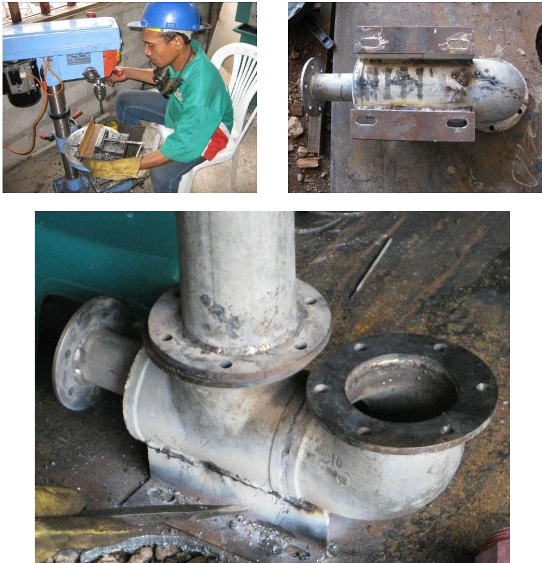
Figure 31: Supports on pump body
