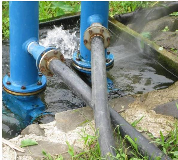
Delivery pipes are straight: flow is linear
