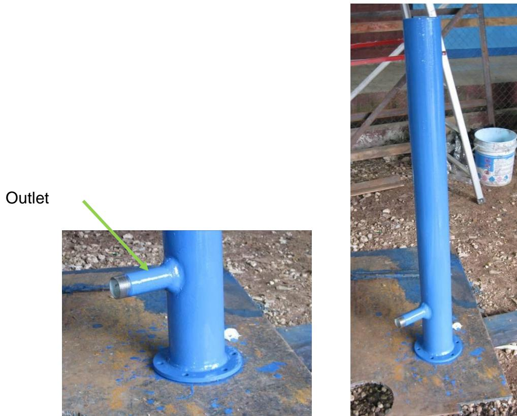
Figure 15: Air vessel
