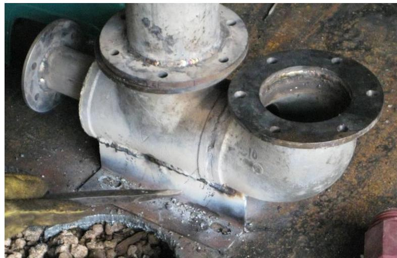
Figure 12.b: Pump body with supports, flanges and reducer
