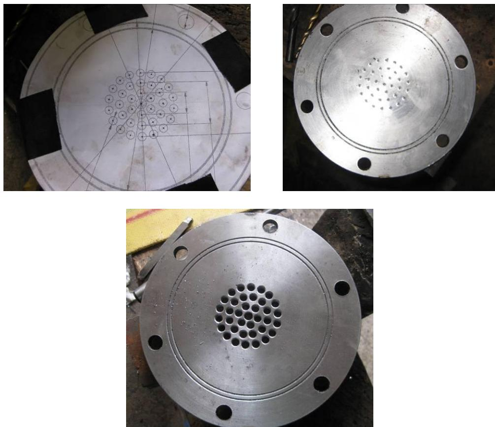
Figure 33: Delivery valve manufacture
