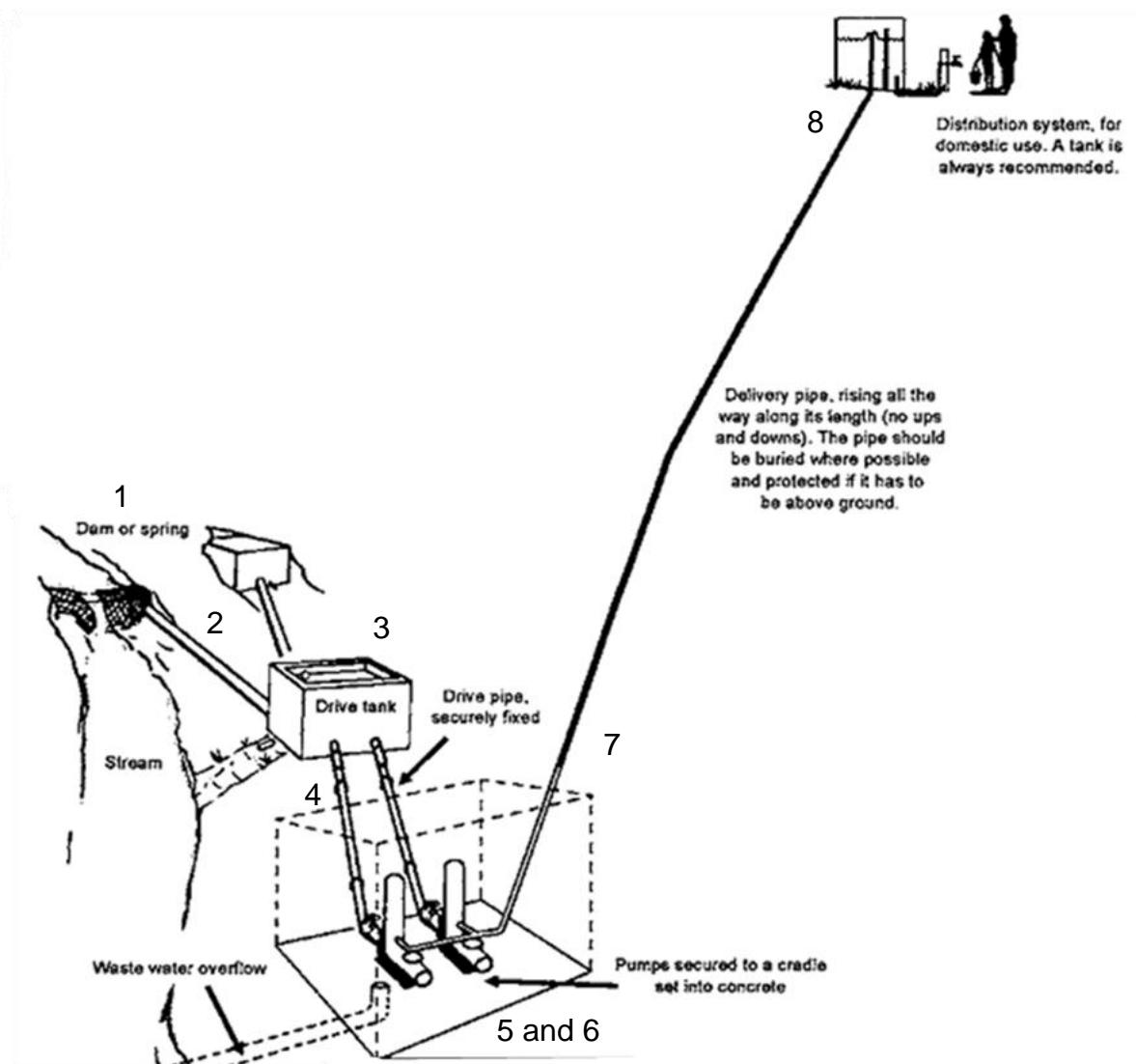
Figure 4: Hydraulic Ram Pump System
