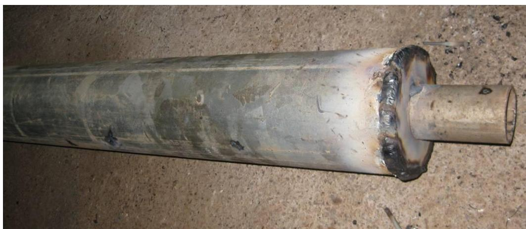
Figure 38: Manufacture of the air vessel
