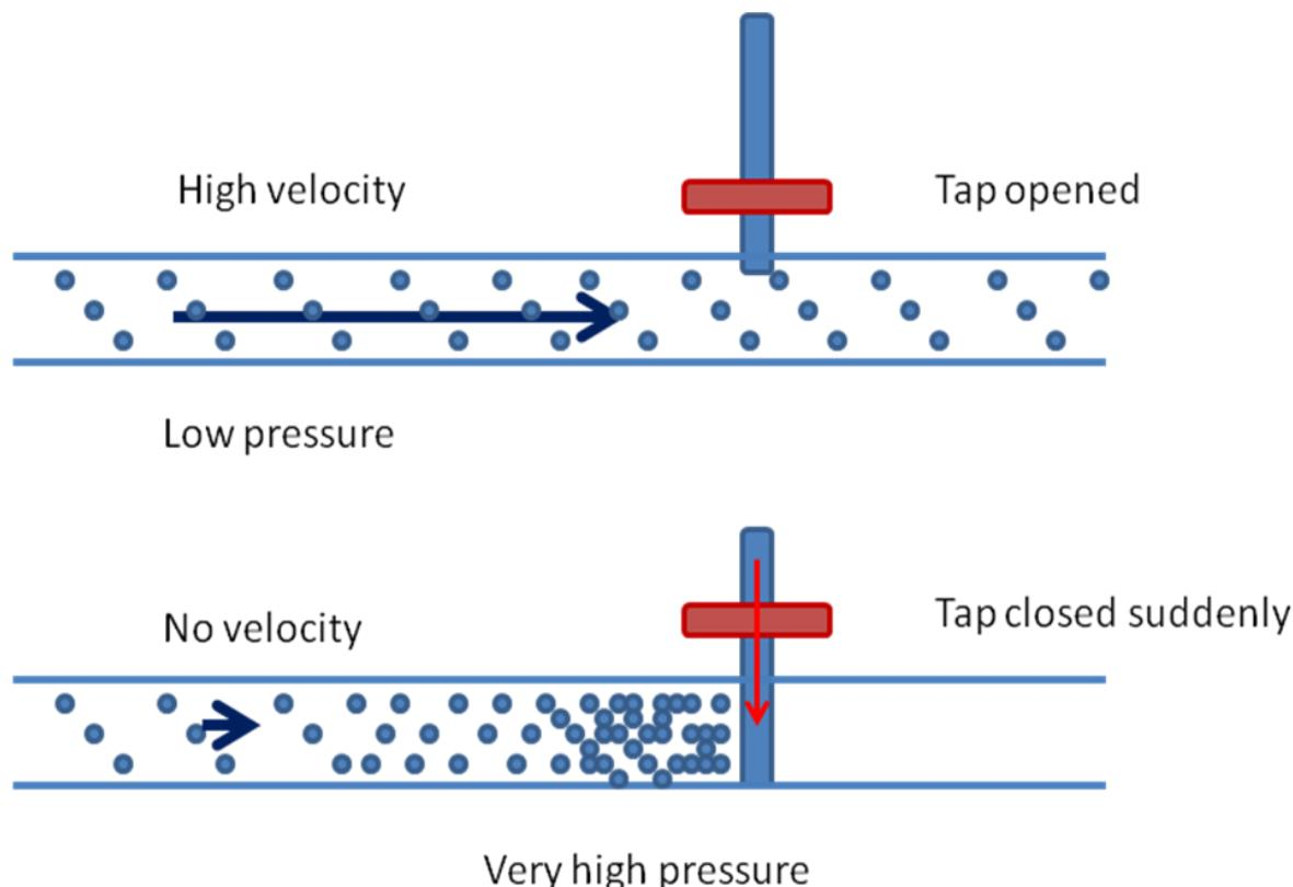
Figure 2: Water hammer effect
