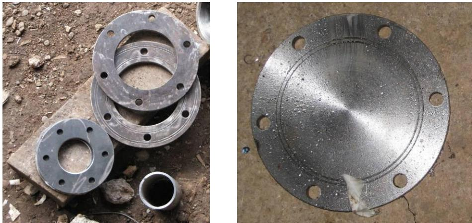
Figure 29: Flanges, plates, reducer, and top of air chamber manufacture
